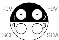
Probe's power supply pin assignment "cable view"
